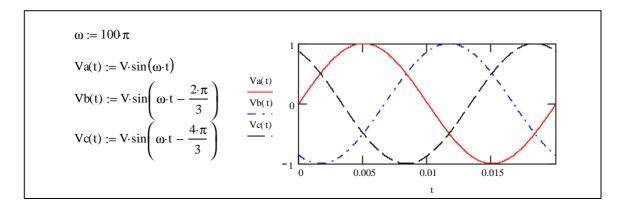
The normal domestic and industrial voltages are derived from a 415 V three phase system.
